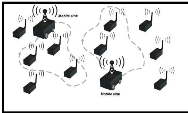
Fig. 2. Illustration of Mobile Data Collectors (MDCs) with mobile sinks
