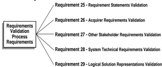
Fig. 1. Validation Process Requirements
