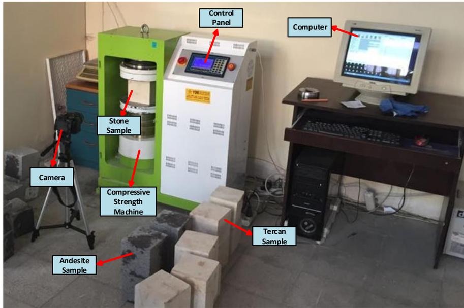
Fig. 7. Experimental setup
