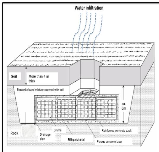
Fig. 2. Concrete Vault Considered in the Calculation of the Computer Code [9].
