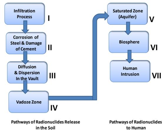
Fig. 3. Different Parts Considered in the GSAD Code
