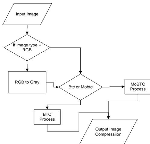
Fig. 1. Flowchart Process Compressing Image with BTC
