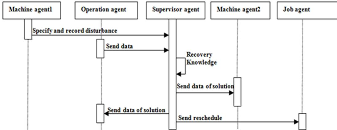
Fig. 4. sequence diagram of mechanism for machine breakdown in case have a learning action
