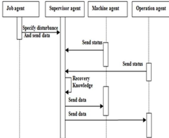
Fig. 6. sequence diagram mechanism for arrival new job in case has a learning action
