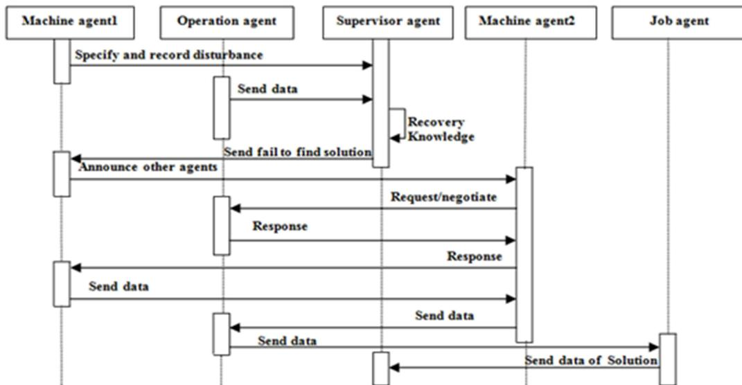
Fig. 5. sequence diagram of mechanism for machine breakdown in case create a new learning action
