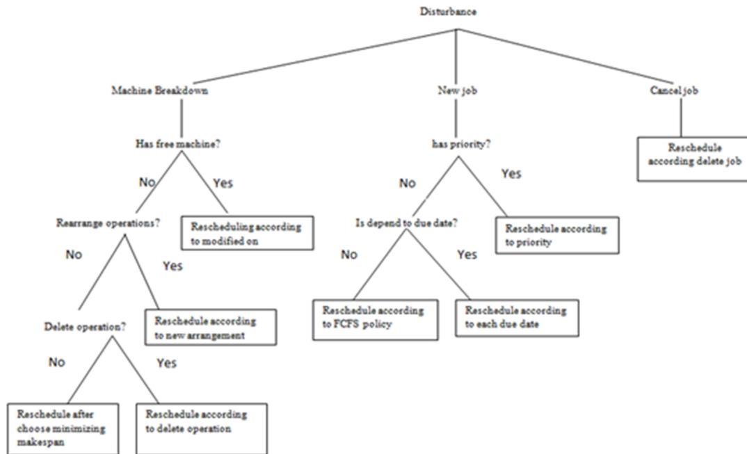
Fig. 3. decision tree for disturbance handling process
