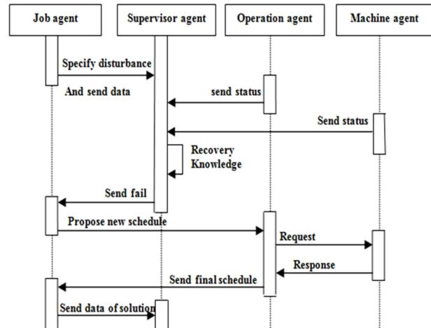
Fig. 7. sequence diagram mechanism for arrival new job in case create a new learning action
