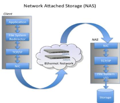
Fig. 4. Network attached storage
