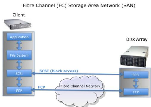
Fig. 2. Fiber Channel Storage area Network
