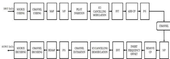
Fig. 4. The OFDM using channel estimation and ICI self-cancellation.
