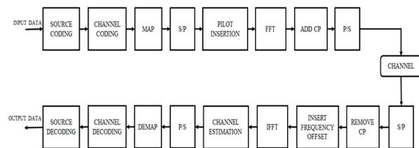
Fig. 1. OFDM block diagram.
